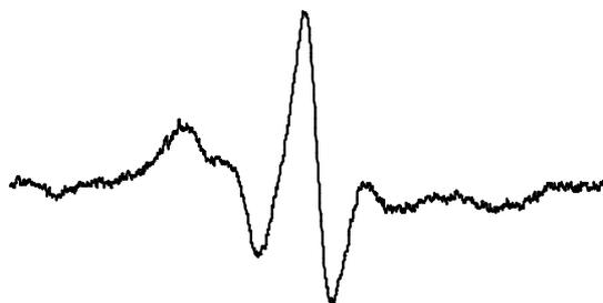
Fig. 27 Anisotropic ESR-spectrum of a spin labelled fatty acid incorporated into liposomes. (*MiniScope MS100*: Scan time 60 s, scan 10 mT, 9.4 GHz).
