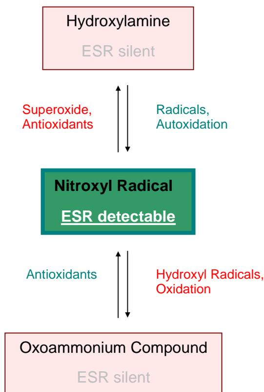
Fig. 5 Reactivity of hydroxylamine spin traps.
