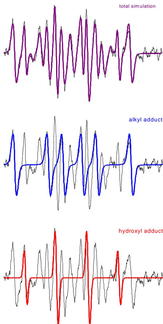
Fig. 15 ESR-spectrum of DMPO-reaction products overlaid with simulated spectra (*MiniScope MS100*: Scan time 60 s, scan 10 mT, 9.4 GHz).
