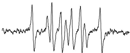
Fig. 17 ESR-spectrum of DMPO adducts after radiation of a porphyrine solution with laser light (*MiniScope MS100*: Scan time 60 s, scan 10 mT, 9.4 GHz).
