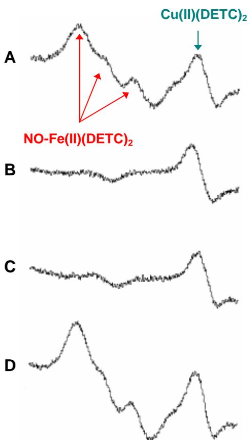
Fig. 1 ESR spectra of strips of rabbit aorta or vena cava (1 cm<sup>2</sup>) incubated with 250 μM colloid Fe(DETC)<sub>2</sub>:
