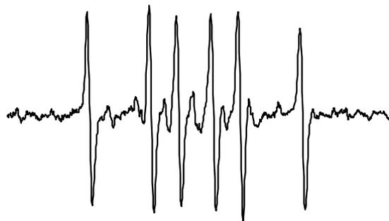
Fig. 35 ESR-spectrum of a DMPO-alkyl adduct which has been produced by massively illuminating a methylene blue solution with laser light for ca. half an hour. (*MiniScope MS100*: Scan time 60 s, scan 10 mT, 9.4 GHz)
