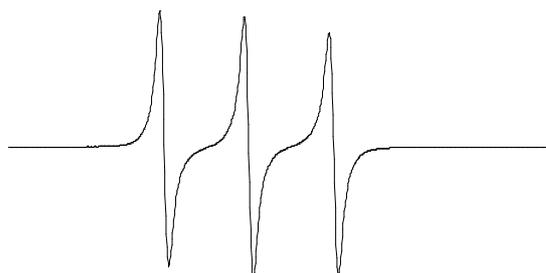
Fig. 30 Spectrum of a stable free radical entailing the NO group of a nitroxyl compound (*MiniScope MS100*: Scan time 60 s, scan 10 mT, 9.4 GHz).
