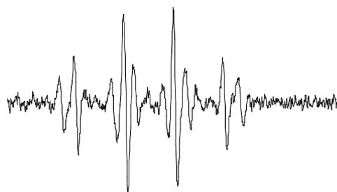
Fig. 38 DMPO, at pH 4 after addition of  $H_2O_2$  (parameters see Fig. 37).
