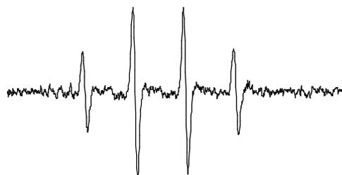
Fig. 37 DMPO, at pH 8 after addition of  $H_2O_2$  (MiniScope MS100: Scan time 60 s, scan 10 mT, 9.4 GHz).
