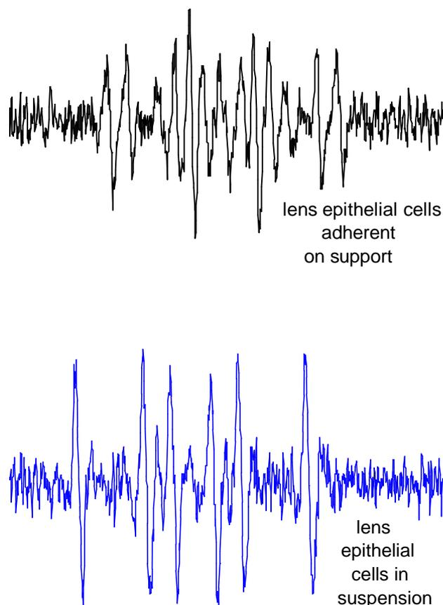
Fig. 16 ESR-spectra of DMPO-adducts formed in a culture of lens epithelial cells. While cells in suspension only show the alkyl adduct (lower panel) those growing on a support have obviously produced additionally hydroxyl radicals which were able to react with the spin trap. (*MiniScope MS100*: Scan time 60 s, scan 10 mT, 9.4 GHz).
