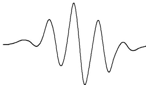
Fig. 14 ESR-spectrum of an irradiated alanine powder sample. (*MiniScope MS100*: Scan time 11 s, scan 15 mT, 9.4 GHz, modulation amplitude 1 mT)
