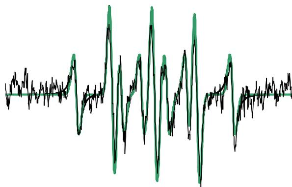
Fig. 23 ESR-spectrum of control roots, fitted simulation superimposed (parameter settings see Fig. 22).
