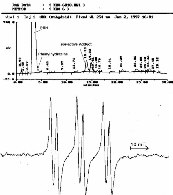
Fig. 29 HPLC chromatogram (upper panel) and ESR-spectrum of the radical containing fraction, recorded on-line (lower panel). (*MiniScope MS100*: Scan time 60 s, scan 10 mT, 9.4 GHz).
