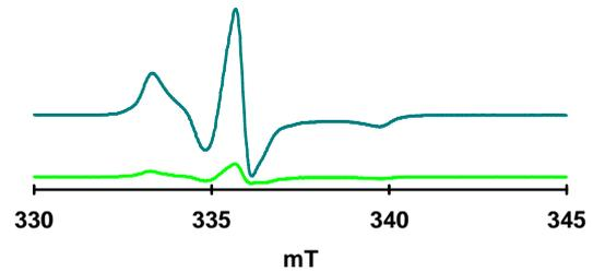
Fig. 19 ESR-spectra of a spin label (TEMPOL) incorporated in to a biologically degradable polyester (PLGA) **before** and **after**  $\gamma$ -radiation (25 kGy, *MiniScope MS100*: Scan time 60 s scan 15 mT, 9.4 GHz). Radiation induced radicals cause spin pairing with the spin label (TEMPOL) and thus decrease the ESR-signal.
