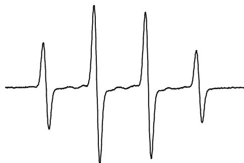
Fig. 36 ESR-spectrum of a DMPO hydroxyl adduct. (100 mM DMPO in phosphate-buffer pH 7.4, Fe(II), H<sub>2</sub>O<sub>2</sub> 1 %, *MiniScope MS100*: Scan time 60 s, scan 7.5 mT, 9.4 GHz).
