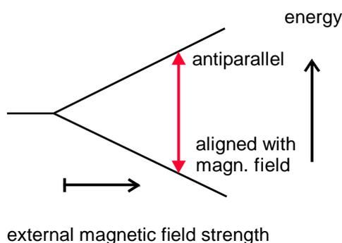
Fig. 31 Energy levels of a single electron in a magnetic field. The difference between these levels increases proportional with the magnetic field strength.
