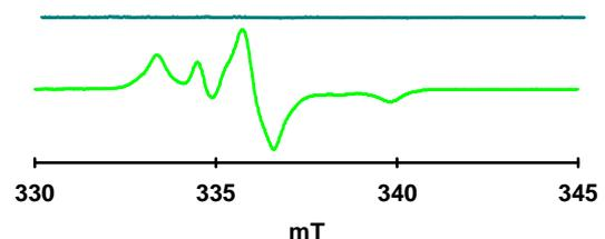
Fig. 20 ESR-spectra of a spin-trap (PBN) in polyester (PLGA) **before** and **after** irradiation (experimental parameters as in Fig. 19).
