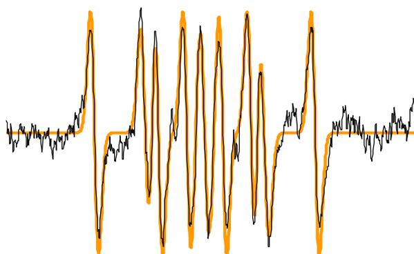
Fig. 22 ESR-spectrum of DMPO-adducts from plant roots exposed to cadmium, overlaid with a fitted simulation (*MiniScope MS100*: Scan time 60 s, scan 10 mT, 9.4 GHz).
