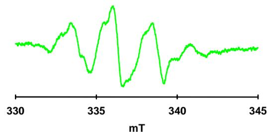
Fig. 21 ESR-spectrum of a polyester (PLGA) containing alanine **after** irradiation (experimental parameters as in Fig. 19).
