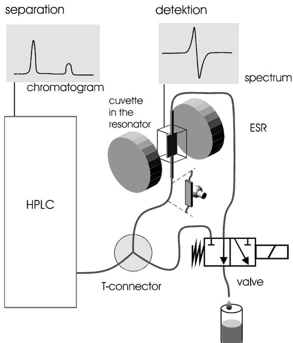
Fig. 28 Combination of a HPLC-device with the *MiniScope MS100* as a radical detector.
