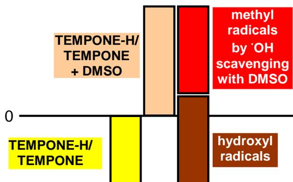
Fig. 7 Calculation of the hydroxyl radical content (dark red) from spin trapping experiments using TEMPONE-H/TEMPONE (yellow) and TEMPONE-H/TEMPONE + DMSO (light brown).
