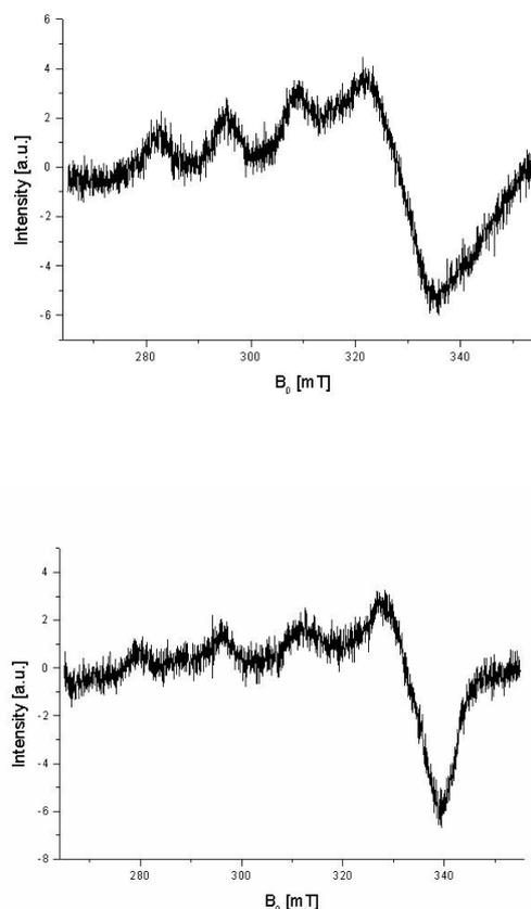
Fig. 25 ESR spectrum of  $\text{Cu}(\text{II})_2\text{Zn}_2$  superoxide dismutase (top) and  $\text{Cu}(\text{II})\text{PuPy}$  (bottom).
